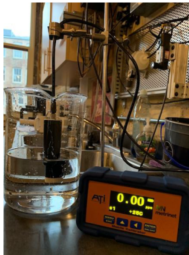
Figure 7: Single M-Node calibration in beaker
